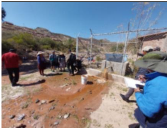
Aforo Pajchapata Lux ( Q=5.40 lts/seg)
